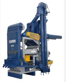
The combined unit CON – pre-cleaner, destoner, huller, repasser and catador – is a compact coffee mill specifically designed to process natural coffees. Its unique combination of cold huller and perforated oscillating screen enables the recovery of 1 to 2% of coffee that is usually lost in conventional machines. The CON's catador separates different coffee qualities that can be directed to different market segments, e. g.: domestic roasters and exporters, with further gains to the user.
