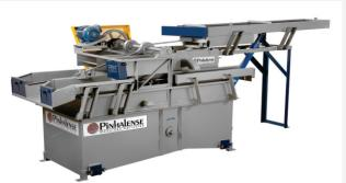
The Pinhalense mechanical siphon LSC separates cherries with different densities and moisture contents in order to dry them separately with savings in full consumption and drying time besides, most importantly, uniform drying and superior cup quality. The mechanical siphon is an environmentally friendly machine that consumes very little water – much less than traditional siphons tanks - , requires no labor and reduces drying time.
