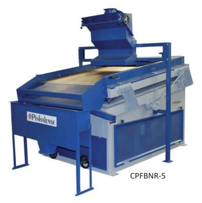
Pinhalense positive-pressure destoners are known to be more precise and to consume less energy than negative-pressure machines that usually cost more. Dust suction devices are available for Pinhalense destoners as for other Pinhalense machines.
