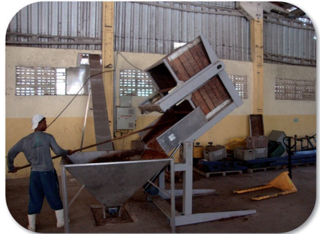
dumper for fermentation boxes
