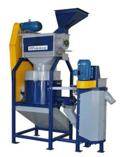
A latest technology Pinhalense mucilage remover is attached to the pulper with the unripe separator in order to make the ECO SUPER 3 a compact machine easy to install, to feed and to operate. This compact setup also saves water as parchment moves directly from the pulper to the demucilager.
