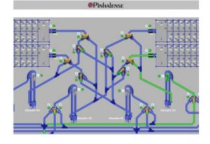
How does SIGA work? Sensors installed in silos and machines, e.g.: elevators and scales, make them "smart". The connection of these sensors to a digital processing system enables control, online management and accounting of operations. These are all reported in digital screens installed in the control center(s) from where operators manage the processing operations and flows.
