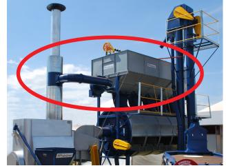
**Heat exchangers** - *investment and fuel efficiency* - Different types of heat exchangers have been used over the years and two types are currently offered in order to adapt to the intensity of use and clients' budgets. The husk feeding system has been improved to increase fuel efficiency and optional equipment to control emission is also available (spark control and after burner).
