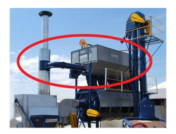
**Drums** - The rotary drums have evolved to accommodate different sizes of batches of coffee to be dried and to increase drying flexibility with the introduction of divided drums of several capacities. As new sizes were introduced, changes in the drums themselves included digital laser punching to ensure a more reliable air flow area and design improvement in the air distribution system.
