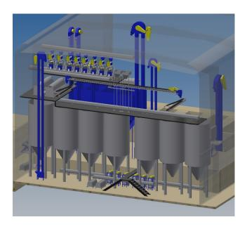
The Pinhalense project portrayed above – one of the largest wet mills in Colombia, currently being assembled – uses dry mechanical transport of coffee and rejects, including coffee pulp, from the feed hoppers to the rotary driers and relies on dry fermentation.
