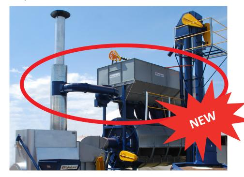
Even though a static drier does not homogenize the moisture of incoming coffee, the SRE rotary drier will perform this task afterward. This will be the case even for lots that arrive with coffee presenting a good dispersion of moisture contents and that cannot be homogenized in a static drier alone.
