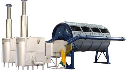
The new driers have two separate heat exchangers, one for each drying chamber of equal volume. This allows for the full flexibility of using the two half-drums in a completely independent manner, for different coffees at different drying stages and with different hot air and temperature requirements. Of course, the two half-drums can also be used with the same type of coffee if the need arises.
